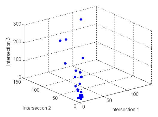
Measure the strength of the linear relationship among the variables in the 3-D scatter by computing eigenvalues of the covariance matrix with the eig function:
