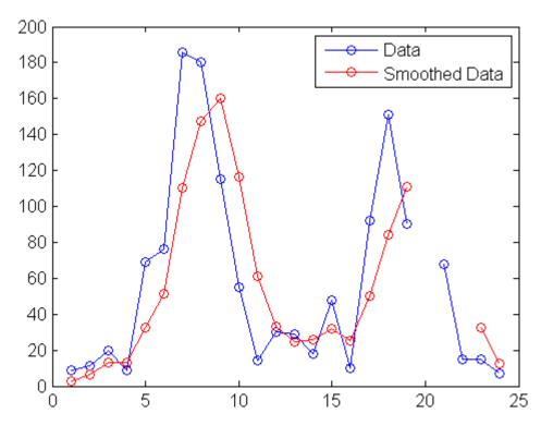
The smoothed data are shifted from the previous plot. convn with the 'same' parameter returns the central part of the convolution, the same length as the data. filter returns the initial part of the convolution, the same length as the data. Otherwise, the algorithms are identical.
